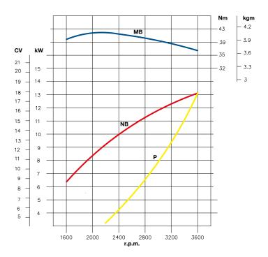
MB – Torque curve (NB curve)
