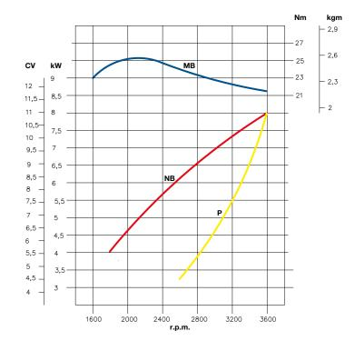
MB – Torque curve (NB curve)
